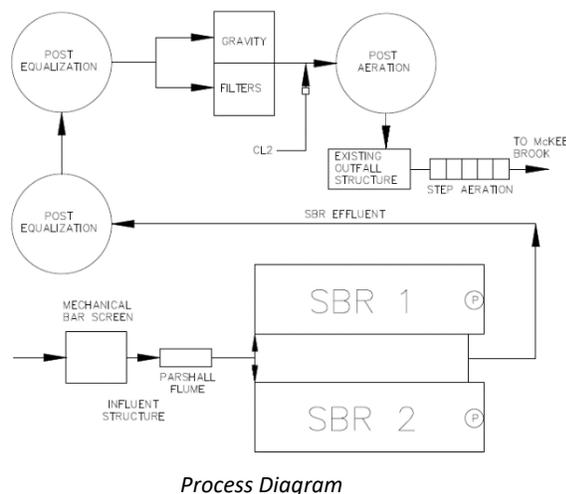
Influent enters the facility through the influent channel structure where it passes through a mechanical bar screen and Parshall flume. Influent then flows to the influent holding tank and then on to the two SBR basins.
